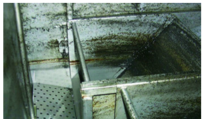
Fig. 3: Adsorptions in the degassing module
