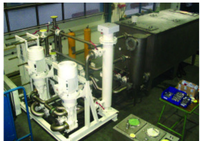
Fig. 2: Oil-lubrication system Lubriflex®, so that everything runs best for the production of the paper money
