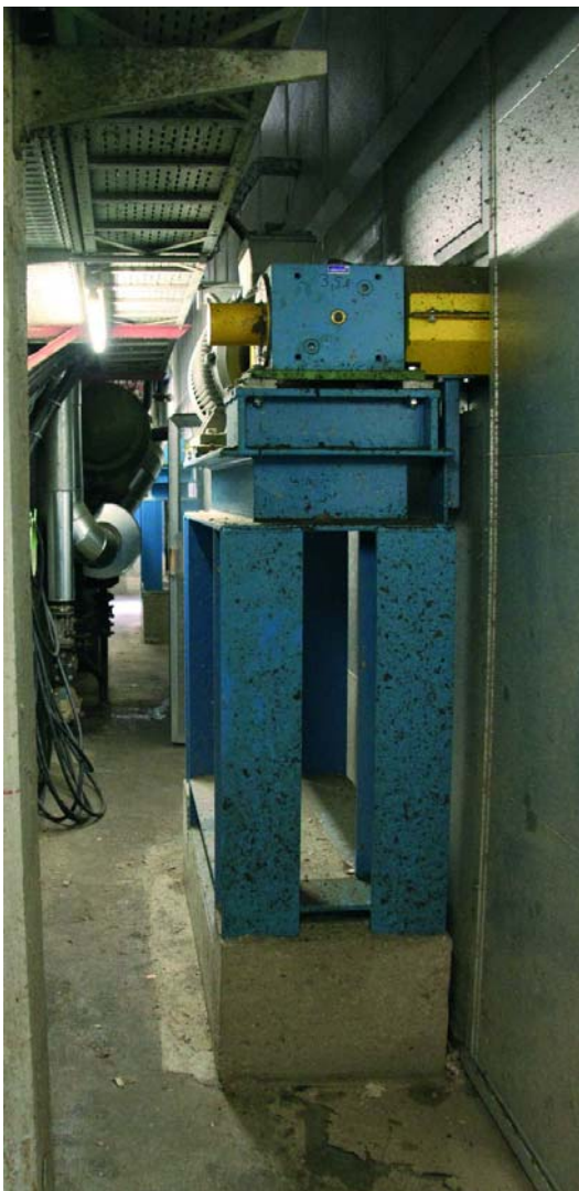
Fig. 12: The installation space behind the PM 1 is very tight. With the FlexoDrive® the foundations and the motors which are out of the hood can be omitted.
