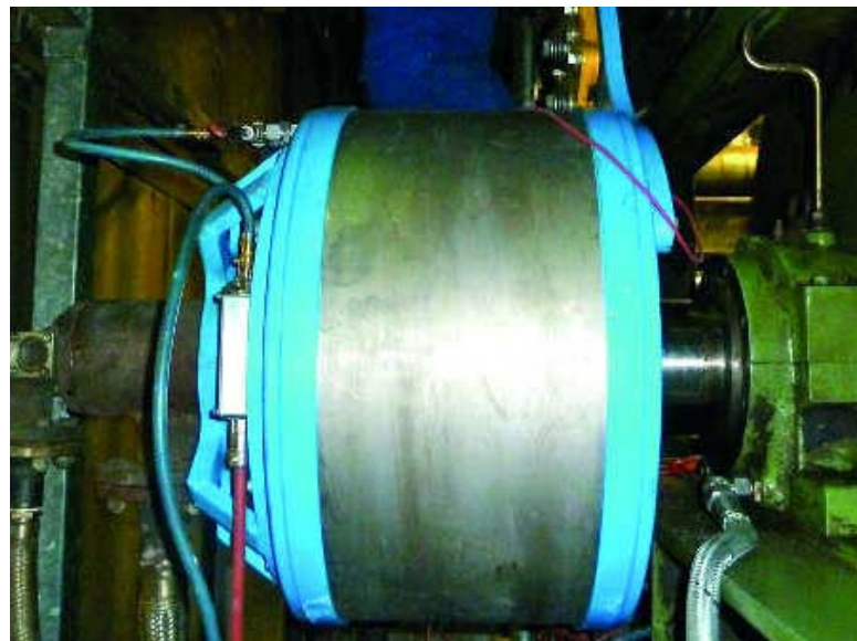
Fig. 11: Even the FlexoDrive® MIDI with 70 kW fits into the construction space!
