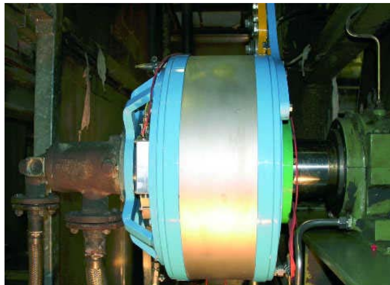
Fig. 10: The FlexoDrive® MINI with 35 kW fits into the construction space!
